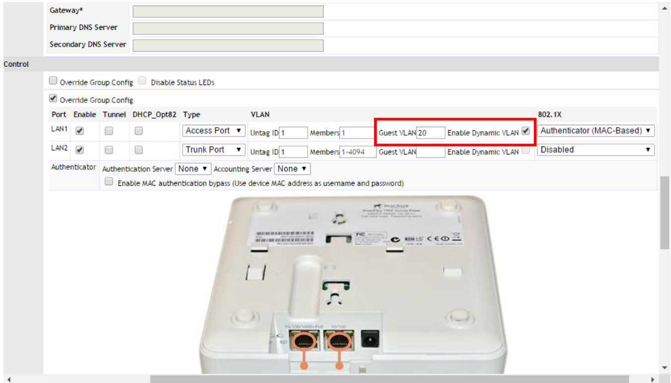
FIGURE 20 Enabling Guest VLAN and Dynamic VLAN on a MAC-based 802.1X Authenticator port
